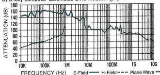
Properly installed Emcor EMI/RFI cabinets will provide the attenuation levels shown on the test data. Any modification to the cabinets as supplied from the factory will vary the specified attenuation results.
